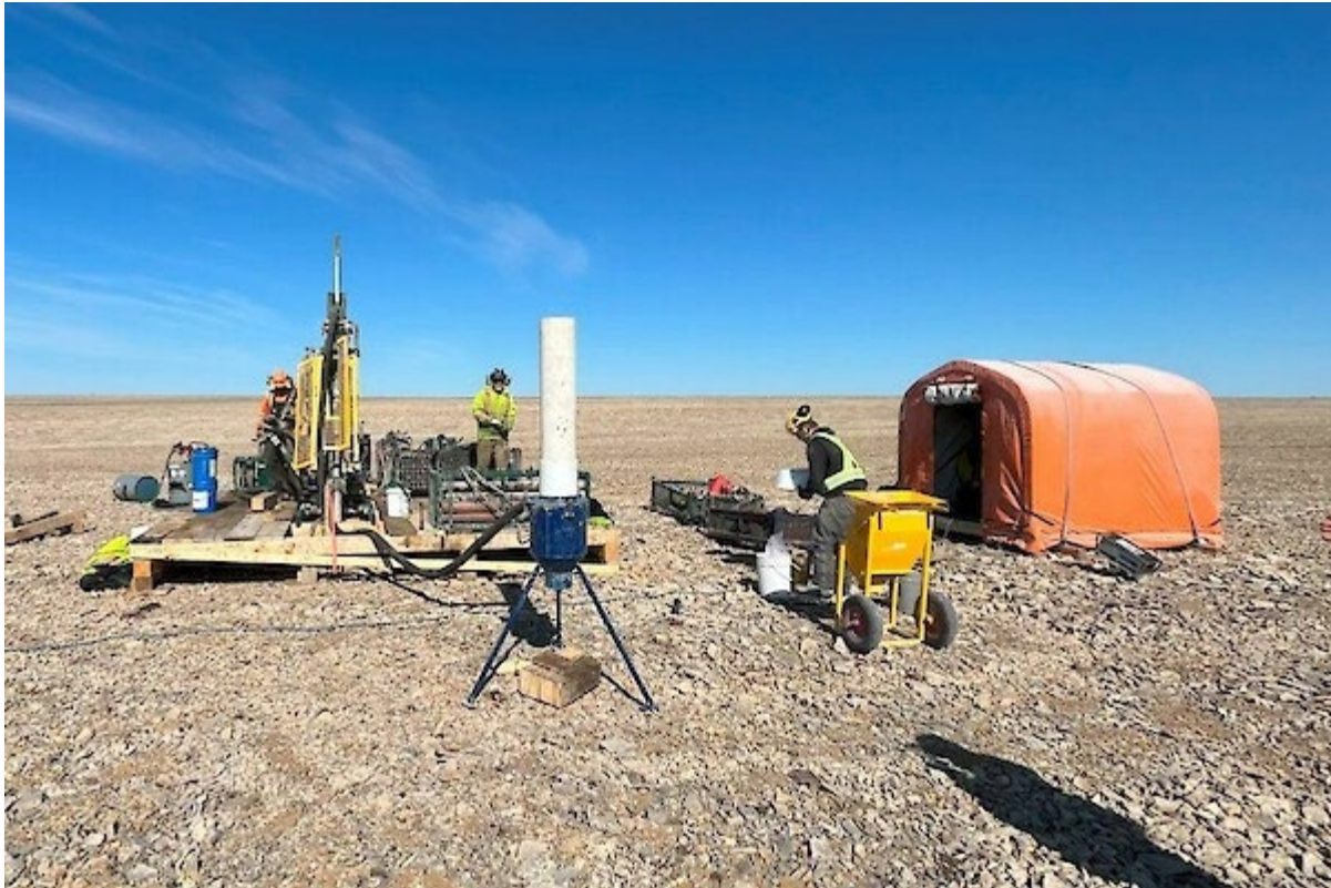
Reverse Circulation resource delineation drilling in 2023 at the 4100N Zone, Storm, Nunavut.
